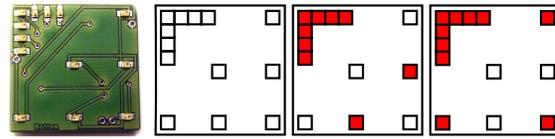
(a) The constructed PCB (b) Left: marker layout; middle and right: two of the  $2^6$  possible configurations
