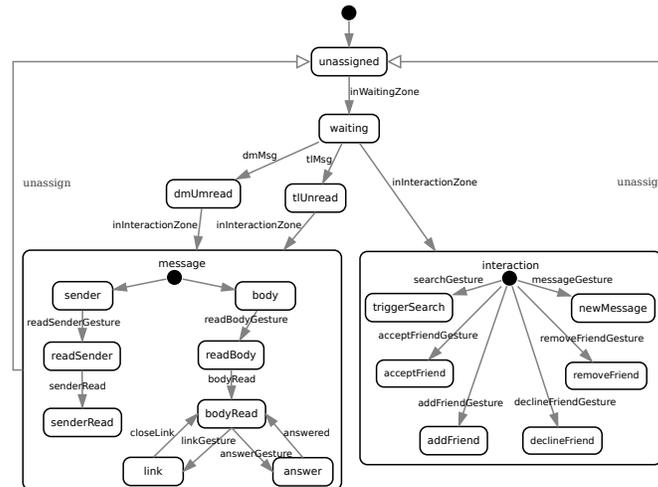
**Fig. 9** State diagram: the implemented finite-state machine. Transition conditions contain message based events (such as *tlMsg*, indicating that a timeline message was assigned) and location based events (such as *inWaitingZone*, indicating that a TAO is in the waiting zone)
